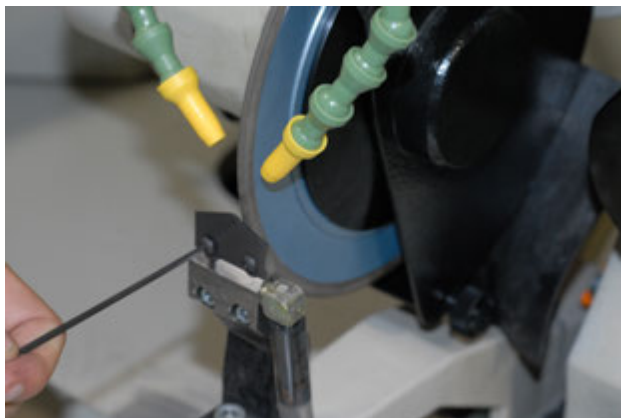
Knife rest and grinding wheel for sharpening blade in a Helicarb cutter on a Weinig Rondamat Grinder or equivalent.
