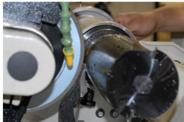
Sharpening blade in Helicarb PowerLock Cutter
