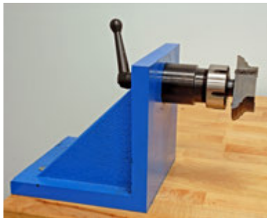
Set-Up Stand shown with collet holder and router bit.
